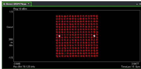
Figure. 8 256-QAM constellation plot at 7115MHz BW20MHz with 10dBm transmit power
