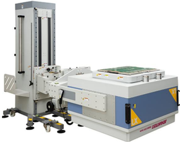
Fig. 11 Example LU set up in ATE (Automatic Test Equipment) 93K environment
