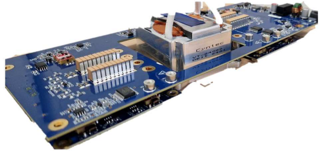
Fig. 6. 7.4 kW prototype: motherboard, planar transformer and the BDS-QDPAK / UDS-TOLT GaN daughter boards.
