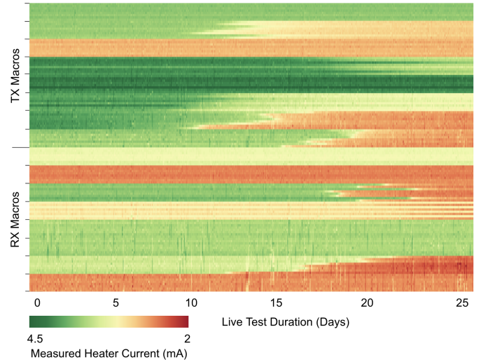
Fig. 4: Real-time current monitoring dashboard of heater degradation on a variant test chip using Grafana heatmaps. Colors are scaled from 4.5 - 2 mA (green to red). Each macro has 8 devices. Each row represents a single heater on the DUT.
